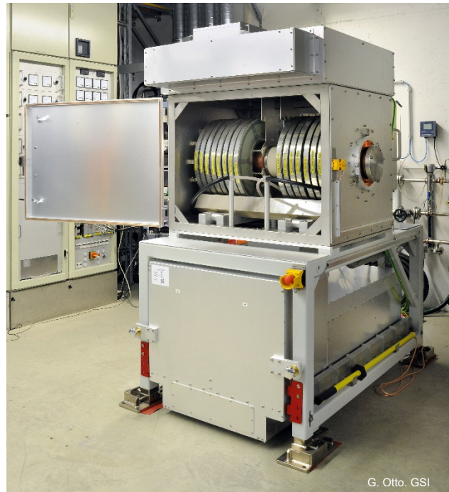
Figure 1: Fully assembled bunch compressor.
